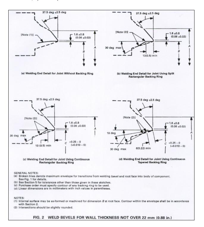
**GWS 1-06 – Weld Joint Design** Attachment 4, Pipe End Prep Details
