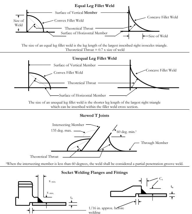
$x_{min.} = 1.4 t_n$  or the thickness of the hub, whichever is smaller, but not less than 1/8 in.  $t_n = nominal pipe wall thickness. C_x = 1.09 t_n$
