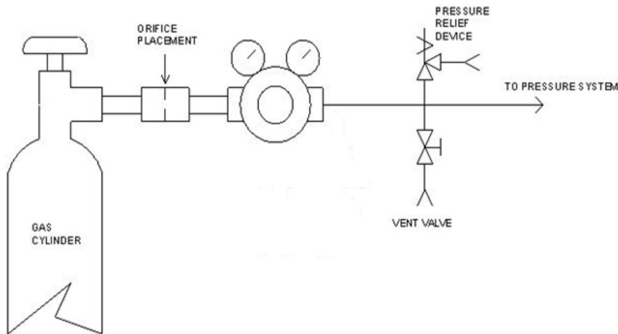
7. *The same orifice may be placed after the regulator, but may present operational issues since the orifice restriction may decrease operational flowrates. In addition, all items between the regulator and the orifice must be suitable for upstream bottle pressure (in the event a regulator fails open). This would include the gauge in the sketch above.*
