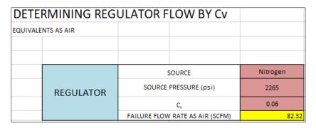
The overpressure protection needs to meet or exceed 82.32 SCFM capacity with a setpoint no higher than the downstream system design pressure of 50 psig. The overpressure protection also cannot exceed 1/4" inlet size to match the size of the connecting system.
