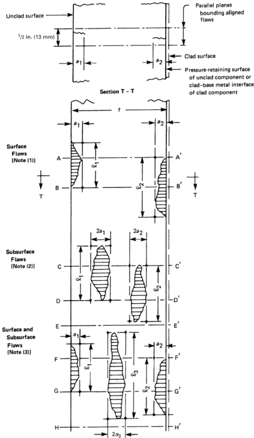
GENERAL NOTE: The flaw depth dimensions  $a_s$  and  $a_e$  are the allowable flaw standards for surface and subsurface flaws, respectively.
